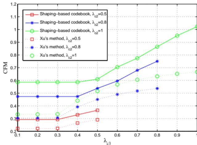
**Figure:** CFM comparison with suboptimal 3 × 3 precoder with 16-QAM in [6], and  $\Sigma = \text{diag}([1, \lambda_{c2}, \lambda_{c3}])$
