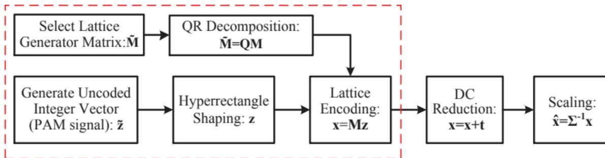
Figure: Flow chart of shaping-based codebook construction
