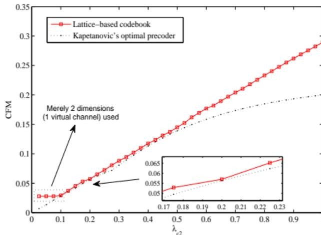
**Figure:** CFM comparison with optimal complex  $2 \times 2$  precoder with 16-QAM in [5], and  $\Sigma = \text{diag}([1, \lambda_{c2}])$
